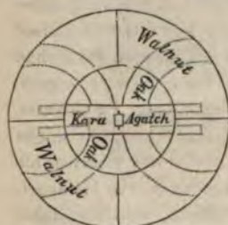
Section of Wheel of Armenian Cart.
