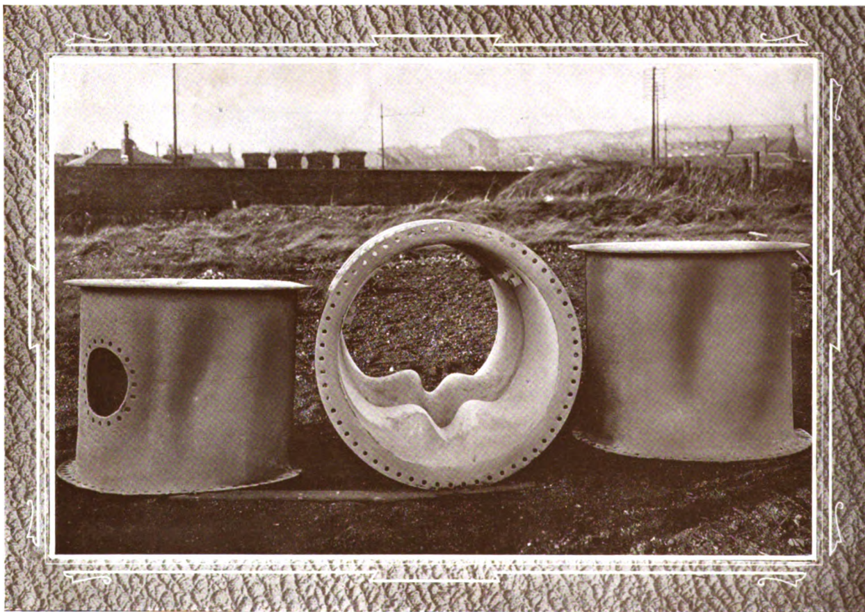
COLLAPSED BOILER FLUES, LOWMOOR IRON WORKS.
