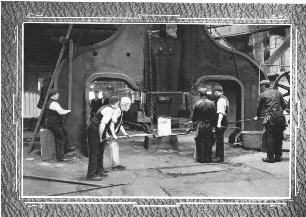
8-Tons STEAM HAMMER, LOWMOOR IRON WORKS. Erected in 1864.
